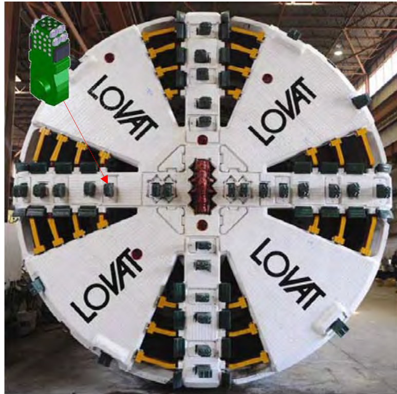
Figure 11 – TBM with tungsten carbide insert, chromium carbide plated ripper scrapers, Brightwater West [68]
